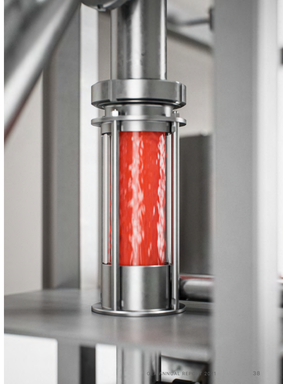
Right: In the process chamber shown, the juice is separated from the mash by means of vacuum.
