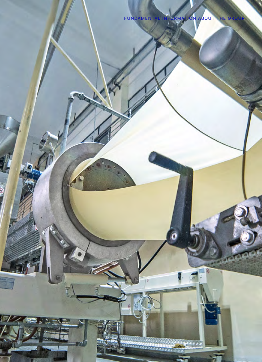
Left: Gelatinized sheet that comes out of the extruder. Below: Ingredients mixture of the Dough
